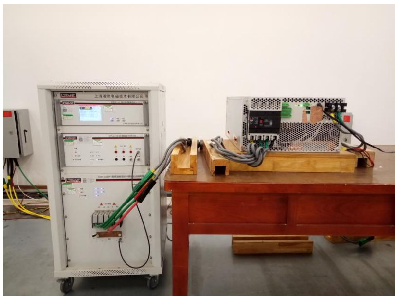
Photograph 6: Set-up for immunity test of fast transient/burst
