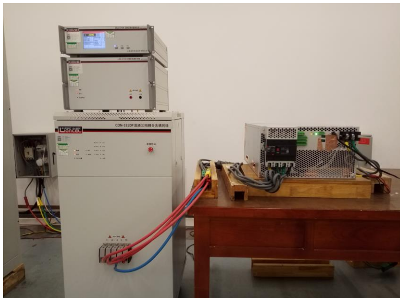
Photograph 8: Set-up for immunity test of surge
