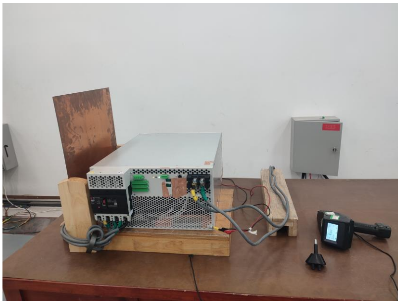
Photograph 3: Set-up for immunity test of electrostatic discharge
