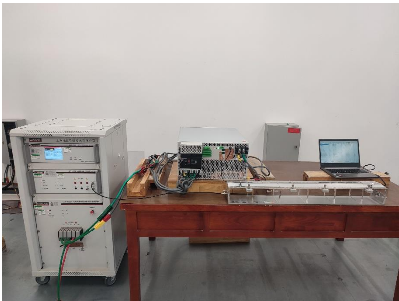
Photograph 7: Set-up for immunity test of Conducted disturbances induced by RF fields
