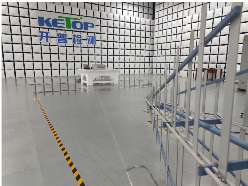
Photograph 2: Set-up for measurement of radiated emission
